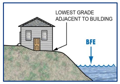
\*Caution: Placement of fill around an existing foundation to increase the LAG could result in non-compliance
