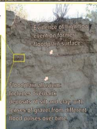
Floodplain alluvial deposits: Layer of rounded gravel and sand, similar to channel bed, indicates sediment was sorted and rounded by water transport.
