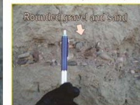
Floodplain alluvial deposits: Layer of rounded gravel and sand, similar to channel bed, indicates sediment was sorted and rounded by water transport.
